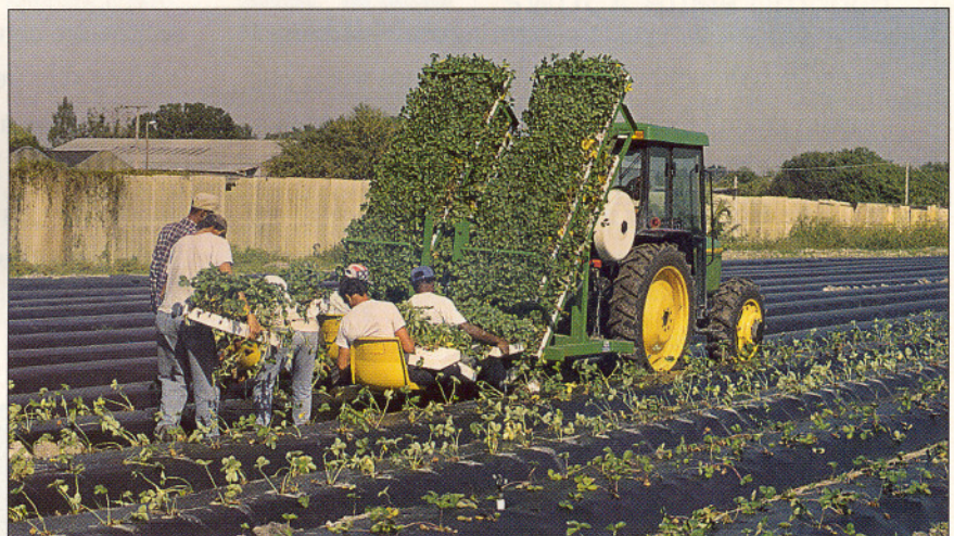
Kennco Manufacturing, Inc. adapted water-wheel transplanter which is used to set strawberry transplants in field at Williford Farms, Ruskin.
