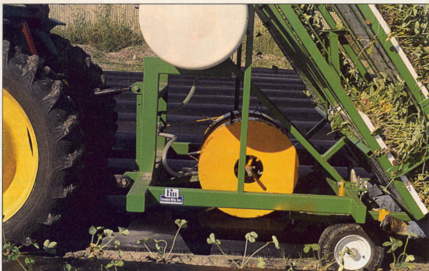
Tank supplies pair of yellow water wheels which irrigate each hole before plant is inserted into the soil, greatly reducing transplant shock.
